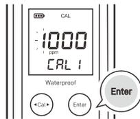
1.4 If necessary, press the **Cal** key to modify the calibration value, press the **Enter** key to confirm and move to the next digit. When the setting is completed, make sure that the displayed value matches the calibration standard.
