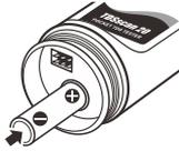
3. Push the electrode into the tester and twist the electrode collar clockwise until tight.
