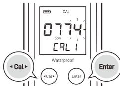
1.5 Press the **Enter** key, the tester begins the calibration. When the reading has stabilized, the display will show **End**. Calibration is completed.
